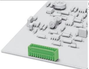
Header, nominal current: 4 A, rated voltage: 80 V, pitch: 2.5 mm, no. of positions: 9, mounting: Soldering
